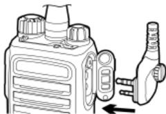
3. Rotate the screw on the accessory plug clockwise until hand tight.
